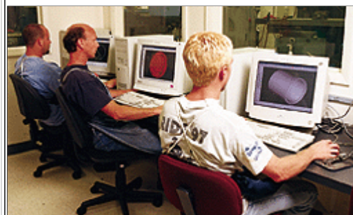
Toolmakers program all of their own toolpaths using Mastercam. This CAM room is dedicated to toolmaking, while another similar room handles modelmaking and prototype toolpath generation.
