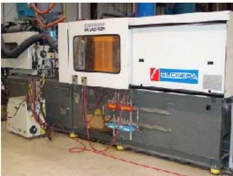
**Electric-powered injection molder**
