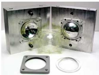
Here are the original two parts of a fuel system product, one plastic and one metal (foreground). Harbec was able to use online collaboration and its Quick Manufacturing Solutions to create the tool in the background. Designers developed a one-piece solution (center) for the Detroit-based customer that reduces assembly time, cost, and leak potential.
