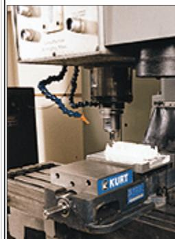
In the model shop, engineering models can be CNC machined from production material and to production tolerances. Other methods of making prototypes include Sanders RP, silicone rubber tooling, and a variety of rapid tooling options.
