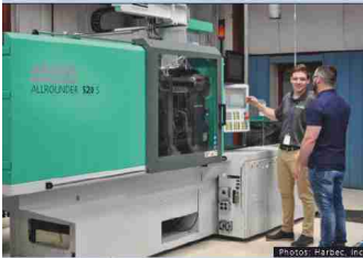
Four of Harbec's five ALLROUNDERS are electrically driven. A hydraulic ALLROUNDER 520 S with the ARBURG energy-saving system (AES – pictured left) is the optimum technical solution for the injection compression moulding of optical lenses (right).
