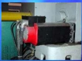
Use of inverter drives and soft starts on all motors 10 hp. and greater saves energy due to more efficient motor starting.
