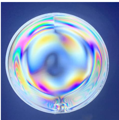
75mm Polymer Lens Commercial Molding
