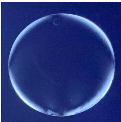
40mm Polymer Lens Zenotherm Molding Process
